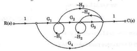
6. Obtain the transfer function using Mason's Gain Formula for the system(APR/MAY 2017)  $H_1 H_2$
