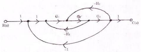
5. Obtain the transfer function using Mason's Gain Formula for the system(APR/MAY 2017)
