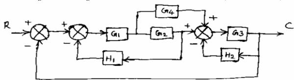
3. For the system represented by the block diagram given below, evaluate the closed loop transfer function, when input R is (i) at Station 1 and (ii) at Station 2 (NOV/DEC 2013) (16 Marks)
