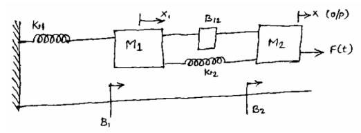
2. Write the differential equation governing the mechanical translational systems shown in the figure. Draw the Electrical analogous circuits. (MAY/JUNE 2015)
