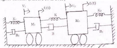
4. Write the differential equation governing the mechanical translational systems shown in the figure. Draw the Electrical analogous circuits. (MAY/JUNE 2013)
