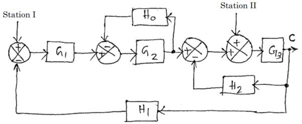
4. Reduce the given block diagram and find the overall transfer function. (APR/MAY 2017) (8 MARKS)
