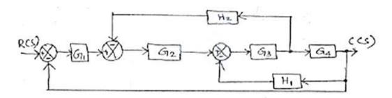
2. Reduce the given block diagram and find the overall transfer function. (NOV/DEC 2014)
