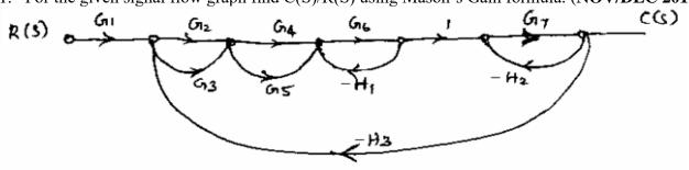
2. For the given signal flow graph find C(S)/R(S) using Mason's Gain formula. (NOV/DEC 2013, APR/MAY 2017)
