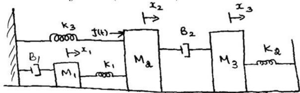
3. Write the differential equation governing the mechanical translational systems shown in the figure. Draw the Electrical analogous circuits. (MAY/JUNE 2013)
