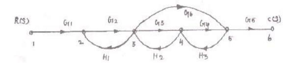
4. Obtain the transfer function using Mason's Gain Formula for the system(MAY/JUNE 2013)
